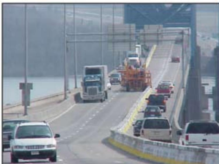
**Figure 2. Moveable Concrete Barrier and Transport Machine**
