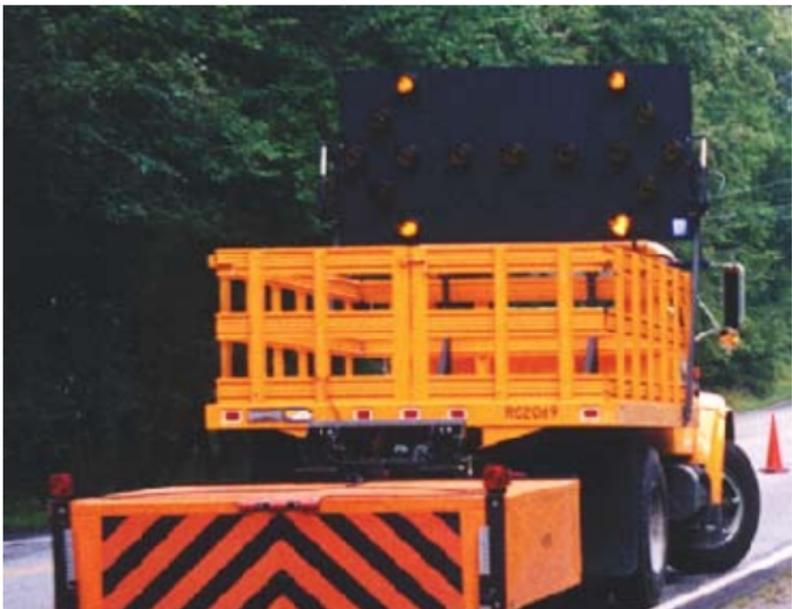
Figure 4. Shadow Vehicle with Attenuator
